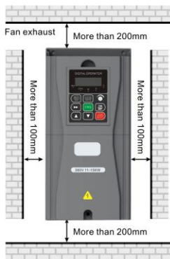
Figure 3-1 Mounting space and distance
